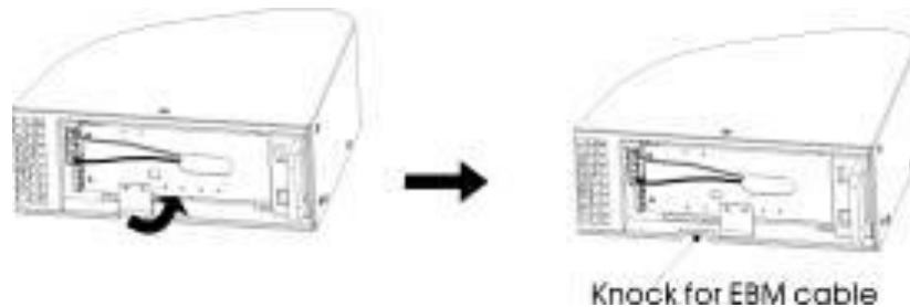
Figure 9 Removing the UPS Cable Knockout
